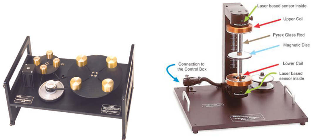
Fig. 2. Schematic of the laboratory industrial plant emulator and magnetic levitation plant.
